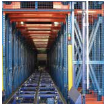
2) Pallet ASRS - Multi Deep with Shuttle System has been designed to accommodate High Density and low SKUs storage capacities.
