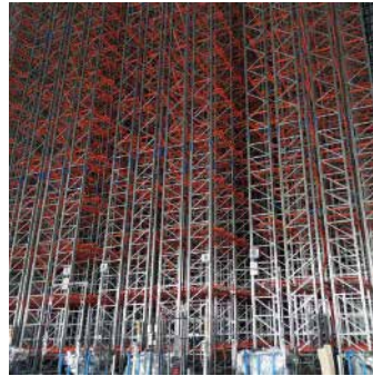
1) Pallet ASRS - Beams with Top Hat for Single or Double storage capacity.
