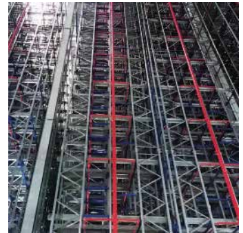
2) Pallet ASRS - Multi Deep with Shuttle System has been designed to accommodate High Density and low SKUs storage capacities.
